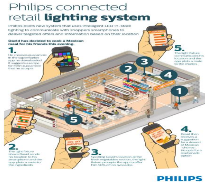
Fig. 9 - Philips Connected Retail Lighting System.
