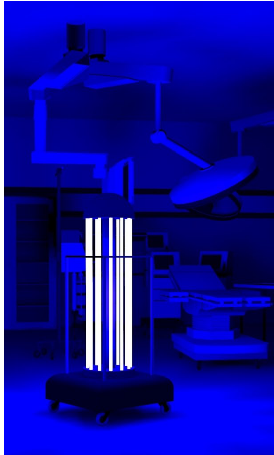
FIG. 1 – Mobile UV-C platform disinfecting a surgical operating theatre.
