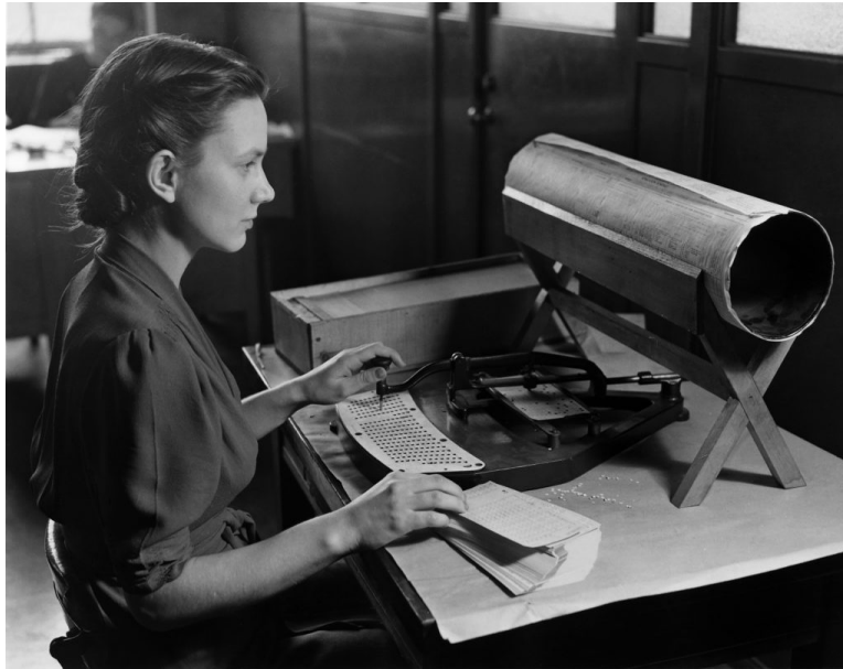
FIG. 1 – IBM Hollerith 80-character punch cards
